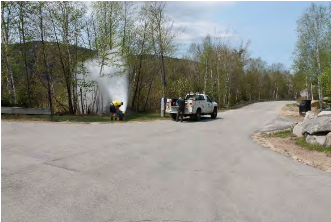
Photo 5-9 View of fire hydrant flow testing as conducted by AWC personnel and their engineering consultant Horizons Engineering.
